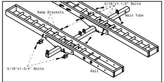
Secure the Rails to the Main Tube and the Ramp Brackets to the indicated Rail using (6) 5/16"x1-1/2" Bolts and (2) 5/16"x1-3/4" Bolts where shown in the figure above. Secure and tighten all Bolts with Lock Nuts (including those from Step 1). The side of each Rail with the empty slot will be where the front tire of each bike sits.
