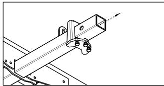
Insert the Anti-tilt bracket onto the Main Tube and insert the carrier into your hitch receiver. After securing the carrier with your hitch pin, push the Anti-tilt bracket against your hitch collar and tighten the 3/8" bolts. Lossely tighten the center bolt first to ensure that it fits just behind the lip of the hitch collar before tightening the side bolts. This prevents the bracket from slipping on rounded hitch collars. After tightening the sides, finish tightening the center bolt.
