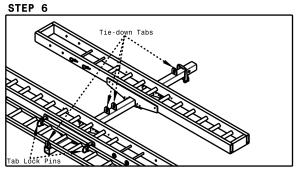
Secure the Ramp on the carrier using the Tab Lock Pins when it is not being used. Secure your bike with straps (not provided) using the Tie-down Tabs as shown.
