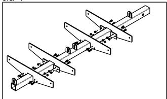
Mount the Rail Brackets to the Main Tube by using the  $5/16"\,x3/4"$  Bolts and Lock Nuts. Do not tighten, leave the bolts lose for now.
