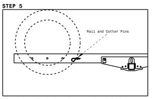
Insert the Rail Pin into the appropriate hole for your specific tire size, such that your bike's tire is supported and resting on the rail. Lock the Rail Pin with the Cotter Pin.
