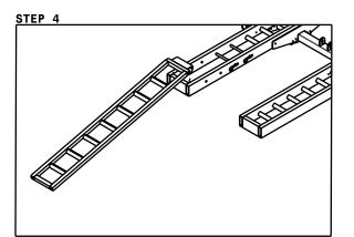
To load your bike, mount the ramp onto the side of the rail as shown.
